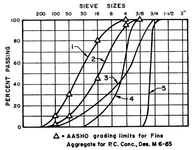
Fig. 2 Grain size curves for five aggregates analyzed in Fig. 1.
