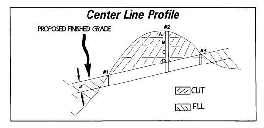
**FIGURE SS-3.** Recommended depth of test holes in cut sections.
