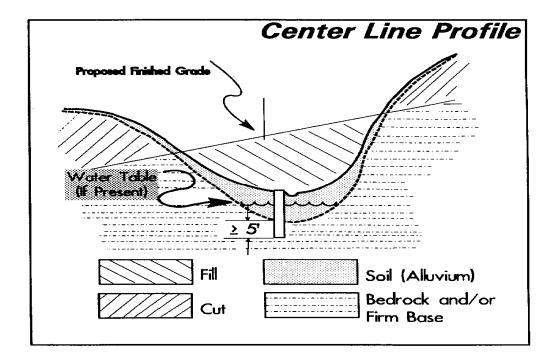
FIGURE SS-4. Recommended depths of test holes in fill.
