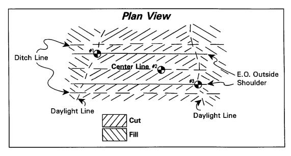
FIGURE SS-1. Recommended location of test holes in the cut section.
